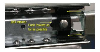
To install the cabinet member or drawer pull the ball retainer all the way forward to contact the plastic ball retainer. Failure to do so may result in damage. Insert the drawer member slowly into the ball retainer guide to reinsert the drawer. Cycle the slide from the fully closed and open positions a few times to recycle the ball cages to complete assembly.
